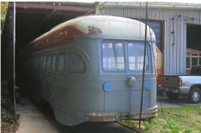
2008 – The car earned the nickname of “gray ghost” once priming was completed. Note that the marker lights have been removed for rechroming. An original style set of “cat’s eyes” taillight lenses were donated and installed. These were just a few of the many small details that were part of this outstanding restoration project.
