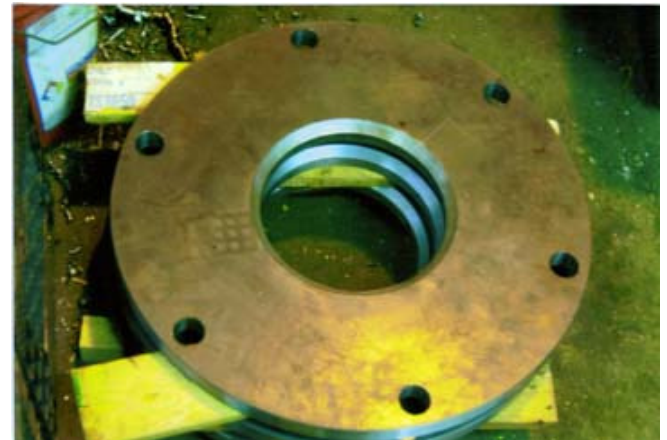
January 2009 – The talented BSM shop crew fabricates new steel wheel spacers (a.k.a. “donuts”) and new bolts to facilitate the regauging of the car to Baltimore streetcar gauge.
