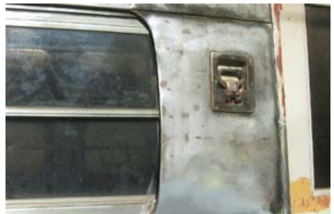
2008 – Great progress! As part of the restoration project, the entire car was stripped to bare steel before additional body preparation work and priming.
