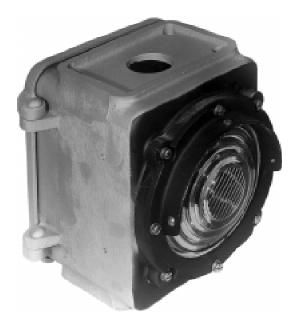
The Model CLS-10D is a rear-access Dwarf Color Light Signal of modular design, allowing multiple units to be easily stacked together. Each unit measures 10 inches in height, 9 inches in width and 8 inches in depth. With dwarf mounting base, a clearance dimension of 19-1/4, 29, or 38-1/2 inches in height is required when mounting 1, 2, or 3 lamp units respectively.
